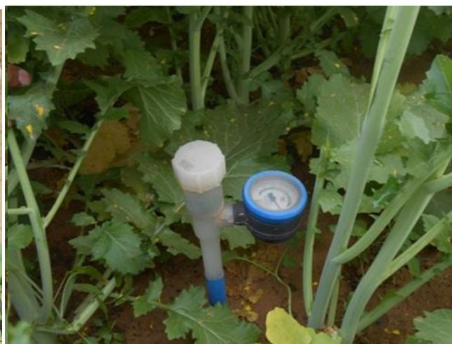
Fig. 3. Tensiometer installed in the plots to measure moisture tension during the crop season
