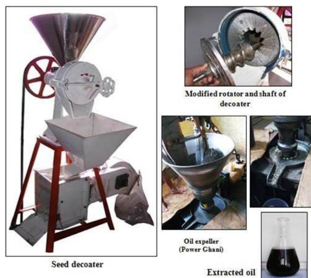
Fig. 2. Seed decoater prototype and oil extraction in power ghani
